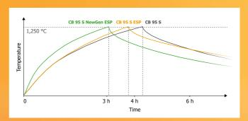
Our test shows: a **CB 95 S NewGen ESP** reached 1,250°C in 3 hours and saved a lot of electricity compared to the **CB 95 S ESP** (3.75 hours) and the **CB 95 S** Standard (4.25 hours).
